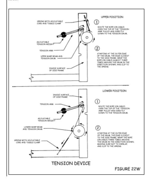
To set the warp tension, move the weight to its rearmost position (next to the wooden pulley). Wind the warp forward slowly, using the ratchet handle on the cloth beam. Continue winding until the weighted tension arm rises and stops when the rope slips on the brake drum.
