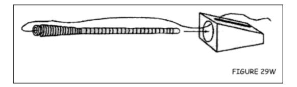
You will begin the winding at the flared cone end. Feed the yarn through the BWG's slot and push the guide toward the cone end. Keep the slot facing you so that you can observe the yarn as it winds onto the bobbin and make any necessary adjustments.
