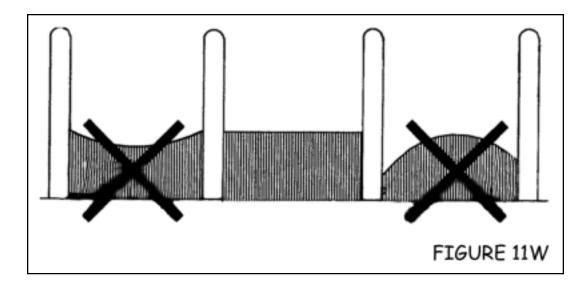
If any of the above is happening, go back and pivot the front reed on the tension box again until you get perfectly flat layers. This is very important, otherwise you will end up having different length threads in one section, since the circumference of the beam within the section is not going to grow evenly. Therefore, you will end up having lots of tension problems.
