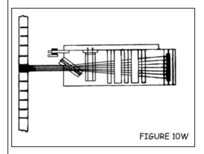
Extra care to correctly center and adjust the width of each warp section will result in more perfect tension while weaving.
