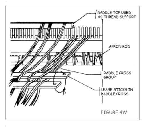
If you are using an AVL raddle with a sliding cover, slide it on after the raddle is threaded and secure it with two or three cord ties so it can't come off. Remove the raddle cross sticks when this is completed.
