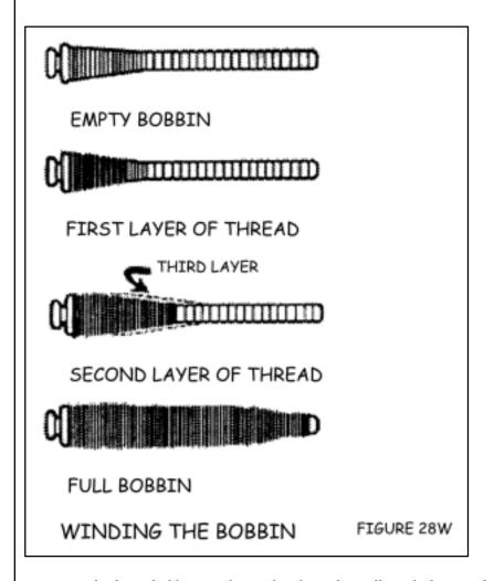
Use a standard size bobbin winder. A hand winder will work, but an electric one is better and some sort of tensioning device is ideal since the thread should be wound very tightly (wearing a heavy leather or fabric work glove will help you to pull the thread tighter).
