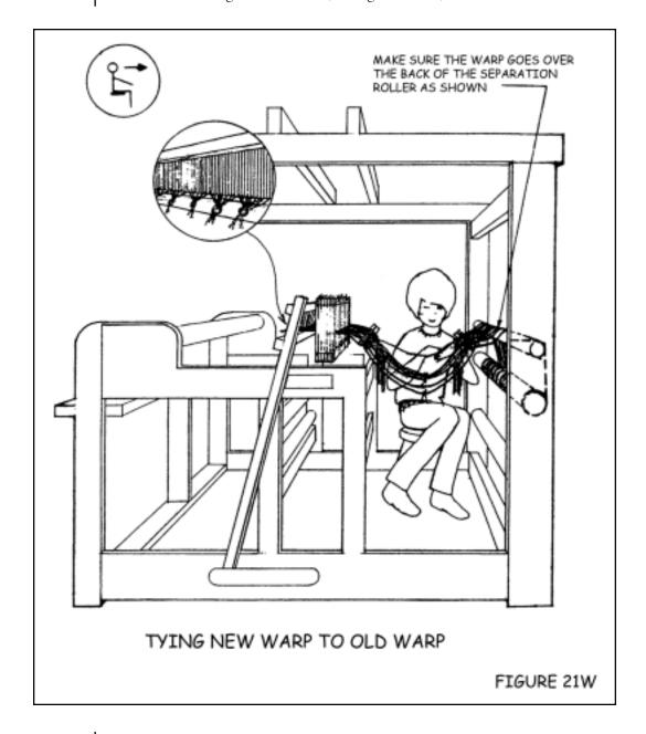
When all ends are tied together, go to the front of the loom and gently pull on the bundles of yarn going through the reed to pull the new warp through the heddles and reed. Then either tie on to an apron or simply wind the ends around the front cloth beam.
