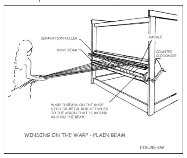
Remember, wind the warp on **tightly** under a lot of tension. This will vary with each warp material, but a good rule to remember is that the tension of the wound on warp must be greater than the tension during the weaving operation. You will need one person to hold a warp under tension on the back and one person to wind the warp on the beam using a handle. The person winding the warp can also insert the paper. For a wide, heavy warp, several helpers may be required.
