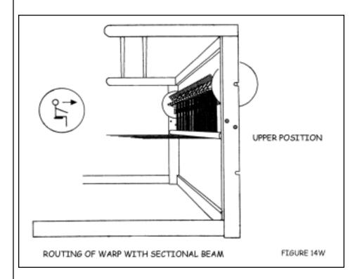
c.) Bring the warp with the lease sticks from the bottom beam around and above the bottom separation roller.
